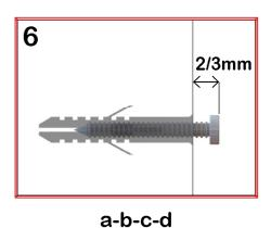
**6.** Drill and insert the screw anchors suited to the type of wall to which the mirror will be fixed (only screws in the case of wood studs).
