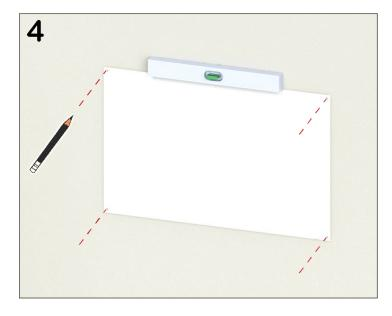
**4.** Tape the paper template to the wall taking into consideration the position of the mounting holes and the mirror edge. With a level, position the template so that it is perfectly level.
